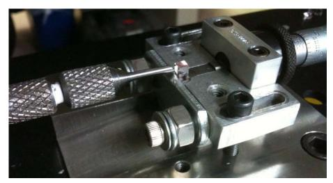
Figure 2. Test fixture set-up for sample fracture strength measurements (phosphate glass sample is shown).
